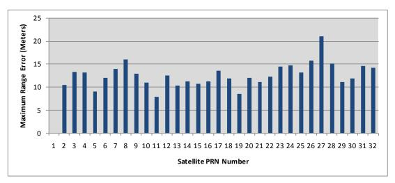
Figure 5-9 Maximum Range Rate Error Per Satellite
