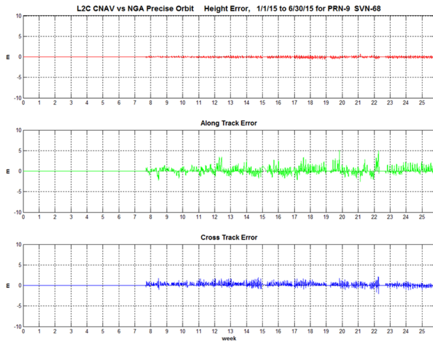
Figure 11-23, Orbit Error PRN-9 (SVN-68) Using L2C CNAV Data
