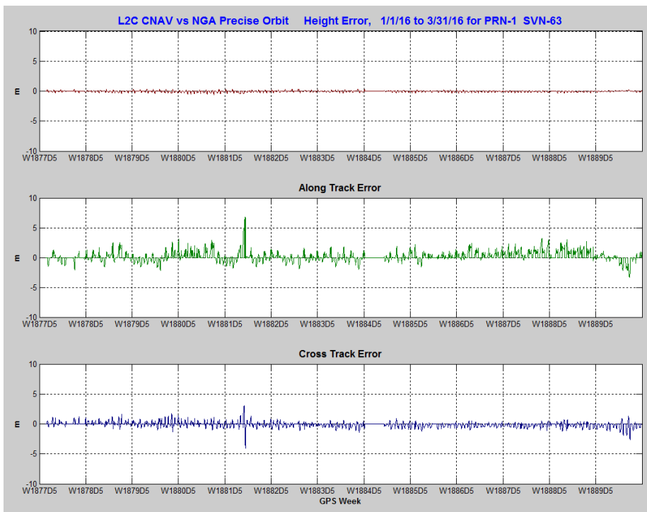
Figure 11-4.2, Orbit Error PRN-1 (SVN-63) Using L2C CNAV Data
