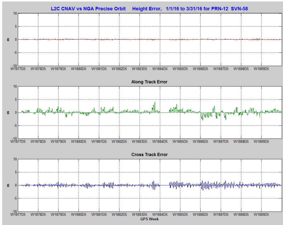
Figure 11-4.19, Orbit Error PRN-12 (SVN-58) Using L2C CNAV Data
