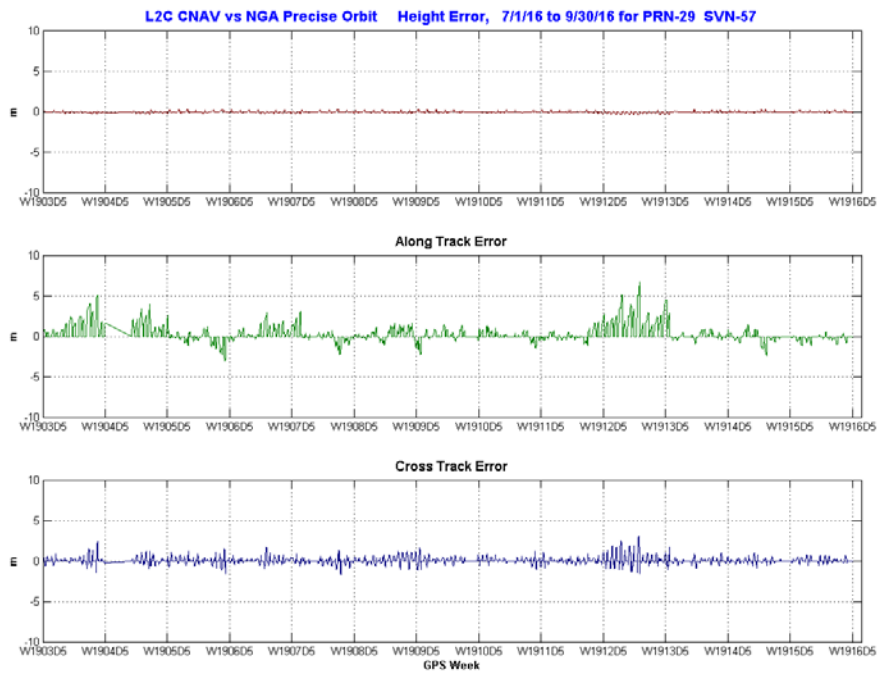
Figure 11-5.44, Orbit Error PRN-29 (SVN-57) Using L2C CNAV Data
