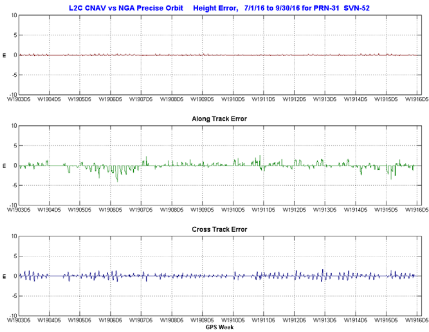
Figure 11-5.48, Orbit Error PRN-31 (SVN-52) Using L2C CNAV Data
