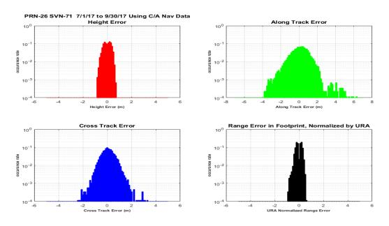
Figure 11-108 Histograms of H, A, C, and Range Error PRN-26 (SVN-71) Using L2C CNAV Data
