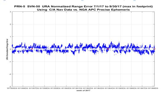
Figure 11-123 Timeline of IAURA Normalized Range Error PRN-5 (SVN-50) Using L2C CNAV Data
