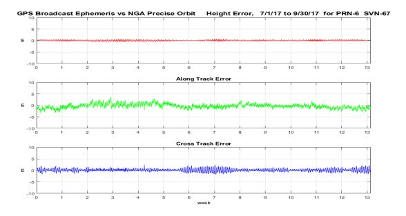
Figure 11-18 Orbit Error PRN-6 (SVN-67) Using L2C CNAV Data
