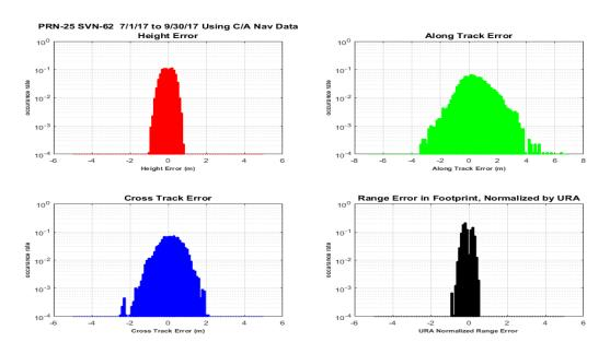
Figure 11-106 Histograms of H, A, C, and Range Error PRN-25 (SVN-62) Using L2C CNAV Data
