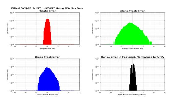
Figure 11-78 Histograms of H, A, C, and Range Error PRN-6 (SVN-67) Using L2C CNAV Data
