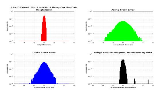
Figure 11-80 Histograms of H, A, C, and Range Error PRN-7 (SVN-48) Using L2C CNAV Data
