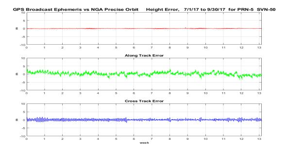
Figure 11-16 Orbit Error PRN-5 (SVN-50) Using L2C CNAV Data
