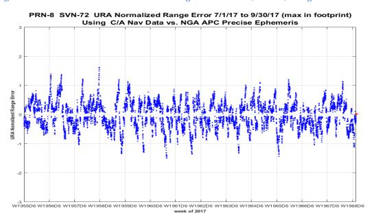
Figure 11-129 Timeline of IAURA Normalized Range Error PRN-8 (SVN-72) Using L2C CNAV Data
