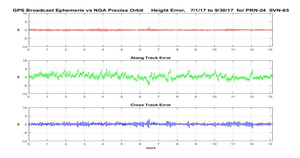
Figure 11-44 Orbit Error PRN-24 (SVN-65) Using L2C CNAV Data
