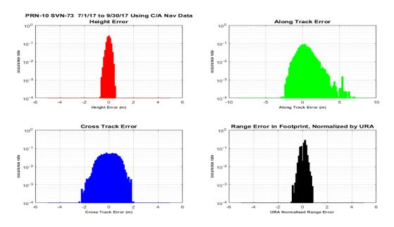
Figure 11-86 Histograms of H, A, C, and Range Error PRN-10 (SVN-73) Using L2C CNAV Data
