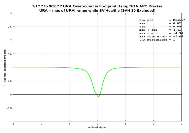
Figure 11-9 IAURA Over-bounding Using L2C CNAV Data
