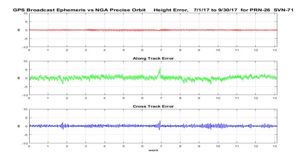
Figure 11-48 Orbit Error PRN-26 (SVN-71) Using L2C CNAV Data
