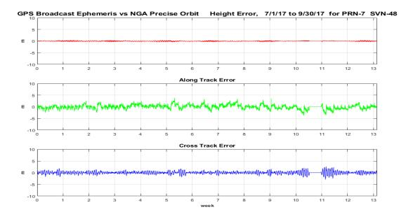
Figure 11-20 Orbit Error PRN-7 (SVN-48) Using L2C CNAV Data
