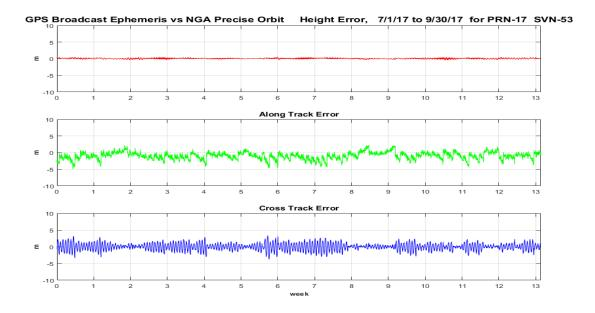
Figure 11-36 Orbit Error PRN-17 (SVN-53) Using L2C CNAV Data
