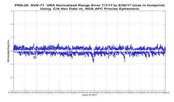
Figure 11-155 Timeline of IAURA Normalized Range Error PRN-26 (SVN-71) Using L2C CNAV Data
