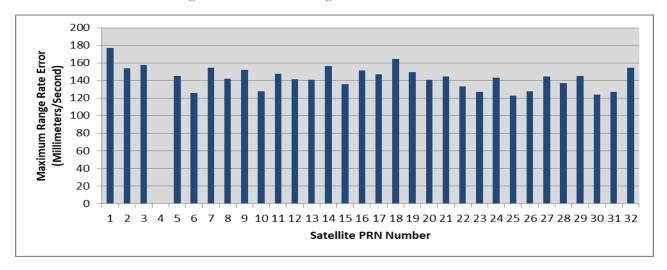
**Figure 5-10 Maximum Range Acceleration Error Per Satellite**
