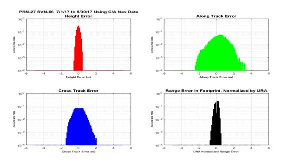
Figure 11-110 Histograms of H, A, C, and Range Error PRN-27 (SVN-66) Using L2C CNAV Data
