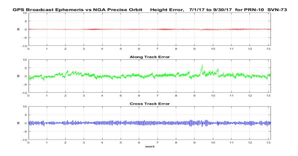
Figure 11-26 Orbit Error PRN-10 (SVN-73) Using L2C CNAV Data
