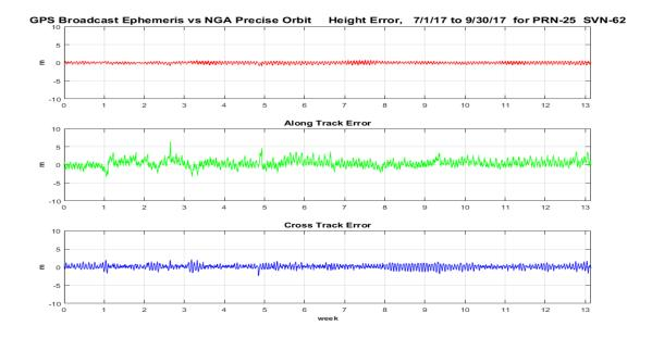
Figure 11-46 Orbit Error PRN-25 (SVN-62) Using L2C CNAV Data
