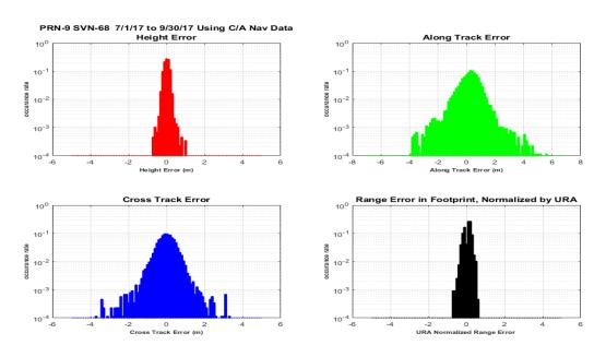
Figure 11-84 Histograms of H, A, C, and Range Error PRN-9 (SVN-68) Using L2C CNAV Data
