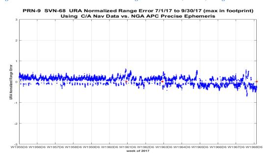
Figure 11-131 Timeline of IAURA Normalized Range Error PRN-9 (SVN-68) Using L2C CNAV Data
