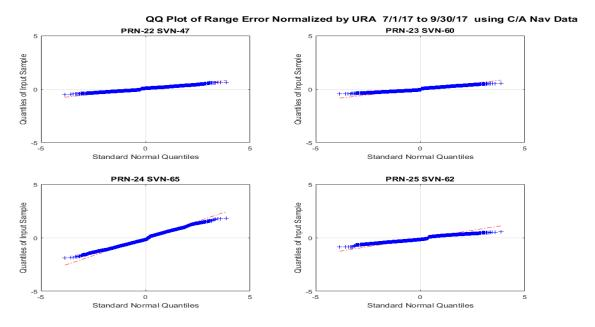
QQ Plot of Range Error Normalized by URA 7/1/17 to 9/30/17 using C/A Nav Data
