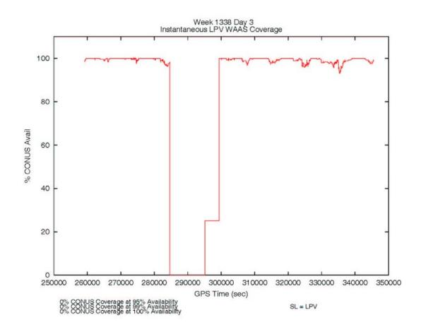
The AORW GEO PRN 122 transmitted a normal message stream after the GUS switch until 284839 GPS time (7:07:09 GMT) when all WAAS receivers lost track of the AORW GEO. At the time of the GUS switch over Santa Puala A (STA-A) ground uplink station (GUS) was primary and Clarksburg was backup GUS with DC master station correction and verification (CnV) the source of WAAS messages for both GUS's.
