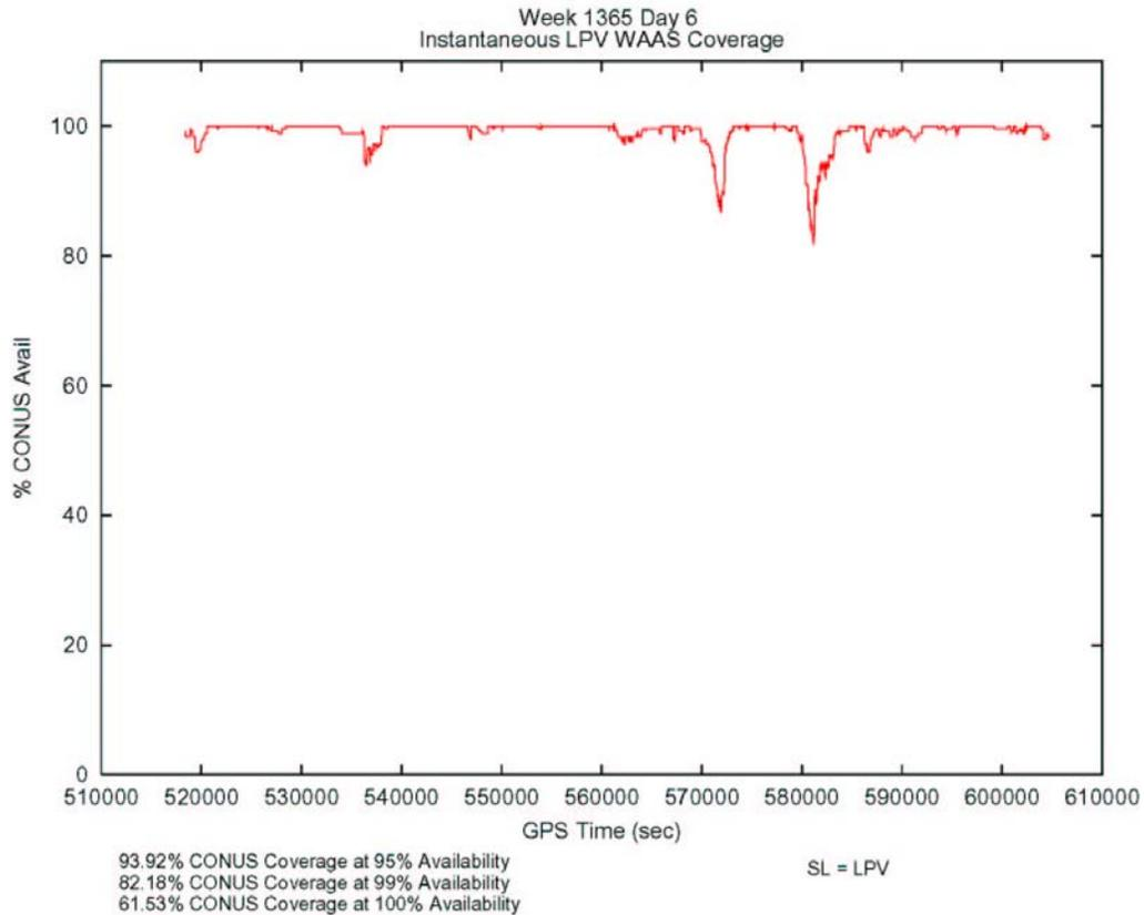
Figure 2 shows that the most serious losses of LPV service over CONUS occurred later in the GPS day. The loss of SV 30 as a PA ranging source is suspected as a likely cause for these drops in availability.
