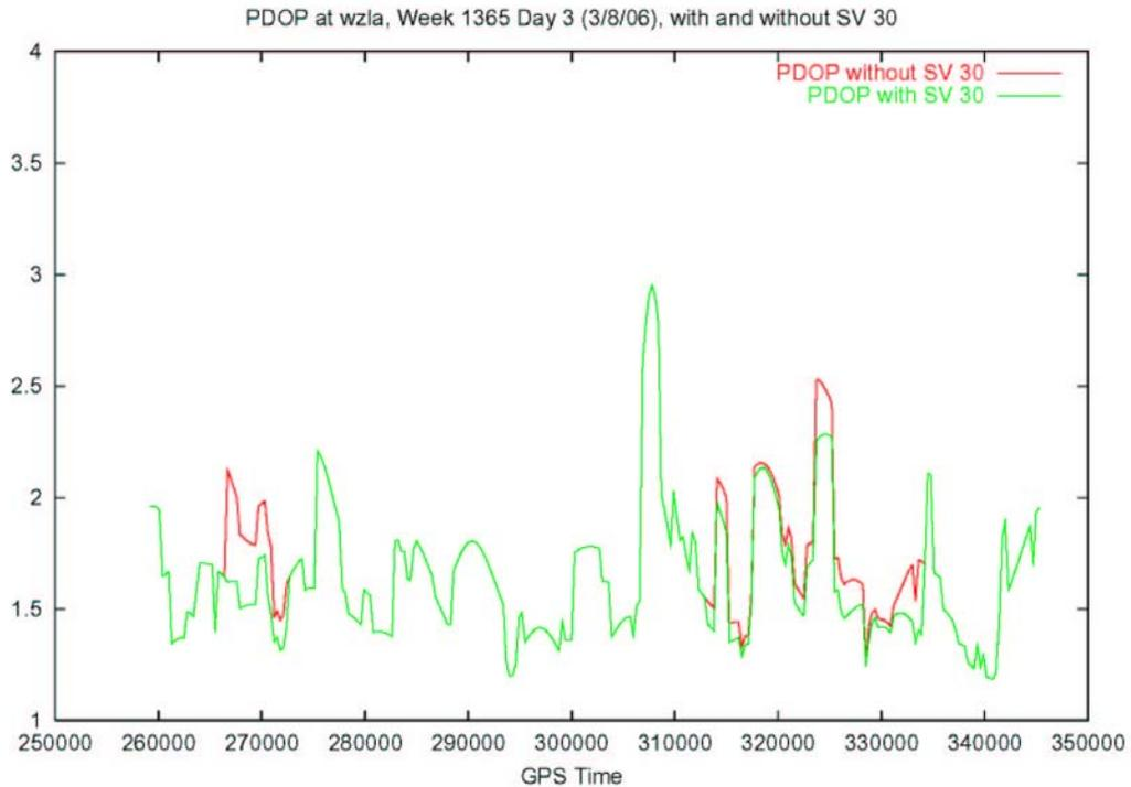
Subtle differences in satellite geometry can have a significant effect on protection levels at a particular location. Simulating the loss of SV 30 on day 3 degraded the geometry for wzla at the same time of day that LPV service was lost on day 6. And again, Figures 3 and 4 show that this is the time of day during which PA ranging via SV 30 would otherwise be available.
