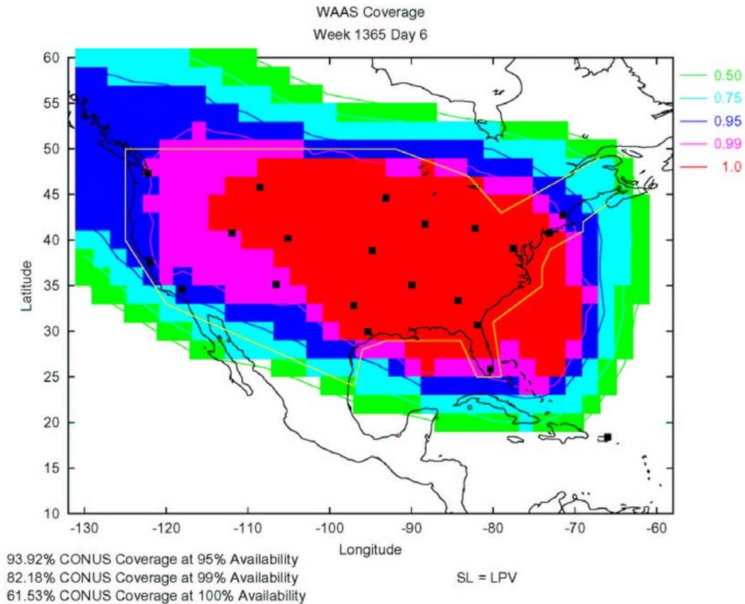
Figure 1 shows where the losses of LPV availability were most significant, namely in the Central Southwestern and Western regions of CONUS. Figure 2 is a plot of instantaneous LPV coverage over the CONUS service volume (30 sec sampling), providing an indication as to when the loss of LPV service occurred over the course of the day.
