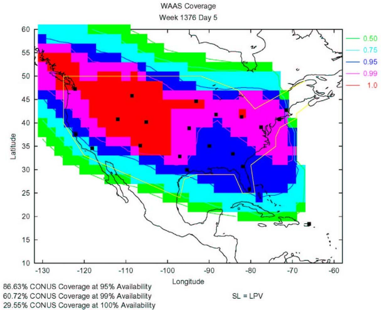
Figure 1 displays a substantial loss of 99% and 100% LPV service across much of the eastern half of CONUS.
