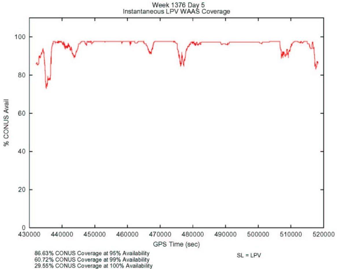
The most apparent loss of LPV service occurred at the beginning of the day.
