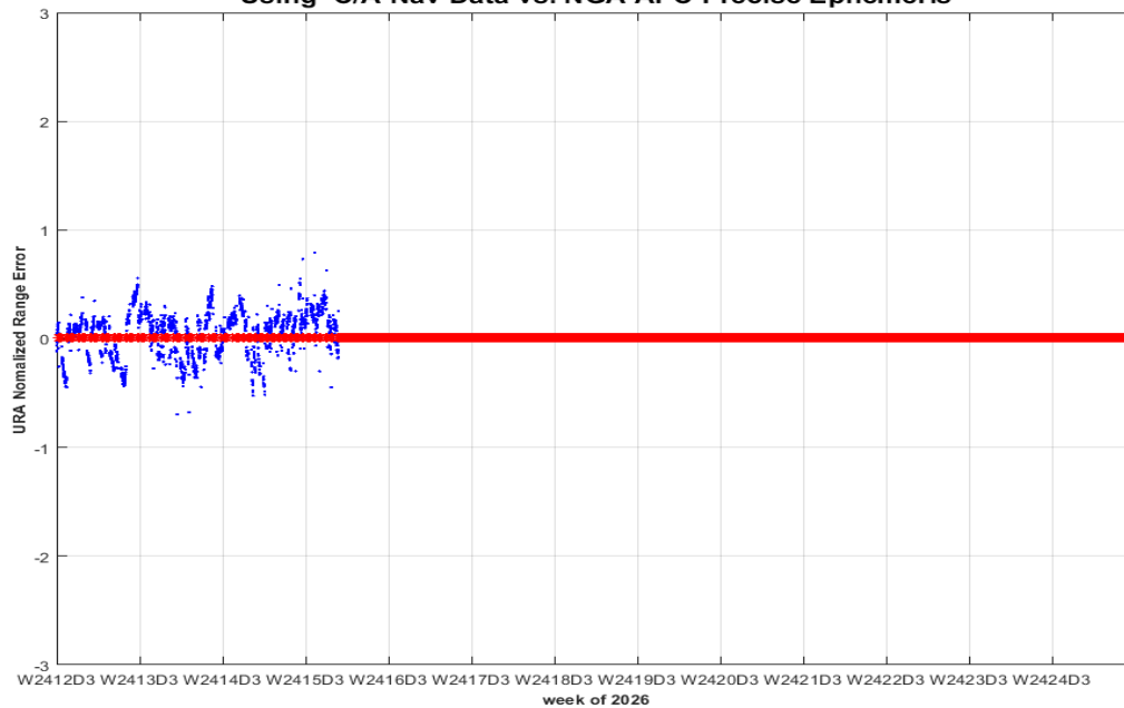
PRN-13 SVN-43 URA Normalized Range Error 04/01/2026 to 06/30/2026 (max in footprint) Using C/A Nav Data vs. NGA APC Precise Ephemeris
